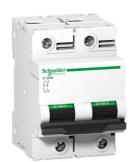
Miniature circuit breaker (MCB), Acti9 C120N, 2P, 80A, C curve, 10000A (IEC/EN 60898-1), 10kA (IEC/EN 60947-2)
