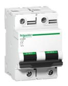
Acti9, Miniature circuit breaker (MCB), Acti9 C120H, 2P, 125A, C curve, 15000A (IEC/EN 60898-1), 15kA (IEC/EN 60947-2)
