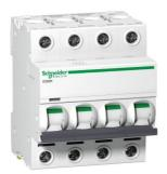
Miniature circuit breaker (MCB), Acti9 iC60H Disbo, 4P, 40A, C curve, 10000A (IEC/EN 60898-1), 15kA (IEC/EN 60947-2)
