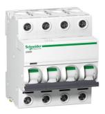
Miniature circuit breaker (MCB), Acti9 iC60H Disbo, 4P, 50A, C curve, 10000A (IEC/EN 60898-1), 15kA (IEC/EN 60947-2)
