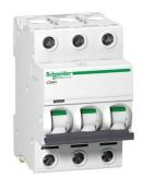
Miniature circuit breaker (MCB), Acti9 iC60H Disbo, 3P, 25A, B curve, 10000A (IEC/EN 60898-1), 15kA (IEC/EN 60947-2)
