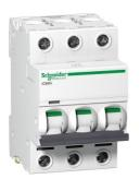
Miniature circuit breaker (MCB), Acti9 iC60H Disbo, 3P, 63A, B curve, 10000A (IEC/EN 60898-1), 15kA (IEC/EN 60947-2)
