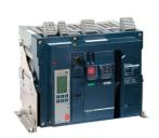
Circuit breaker frame, MasterPact NW32H2, 3200A, 100kA/440VAC 50/60Hz (Icu), 3 poles, fixed, without control unit
